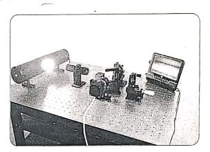
7. Adjust the mirror tilt and position of the camera for clear and sharp circular fringes.
