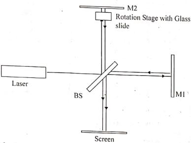
In principle, the method for calculating the index of refraction is relatively simple. The light passes through a greater length of glass as the plate is rotated. The general steps for measuring the index of refraction in such a case is as follows:
