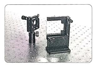
2. Fix the high precision mirror with translation stage ( $M_1$ ) & mirror with coarse movement ( $M_2$ ) in equal distance from the beam splitter.
