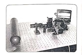
The two beams of a Michelson interferometer interfere constructively when the waves add in phase and destructively when they add out of phase, producing circular interference fringes as a result. With Sodium source the wavelength is given by
