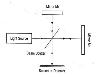
$M_1$  and  $M_2$  are two plane mirrors silvered on the front surfaces. They are mounted vertically on two translation stages placed at the sides of an optical platform. Screws are provided at the back of the holders. Adjusting of which allows  $M_1$  and  $M_2$  to be tilted.  $M_1$  can also be moved horizontally by a micrometer attached to the  $M_1$  holder.
