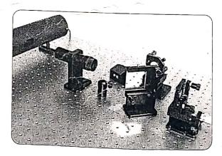
6. Replace the screen with camera. Observe the fringe pattern on the display.
